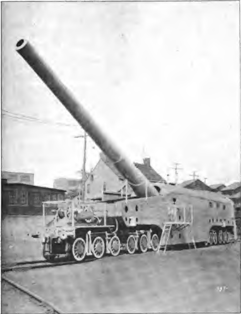
14-INCH, 50-CALIBER AMERICAN NAVY GUN MOUNT, MARK I. 181768—21—22
